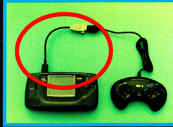
Master Link Connects a Sega controller to Game Gear for 2 player simultaneous game play.
