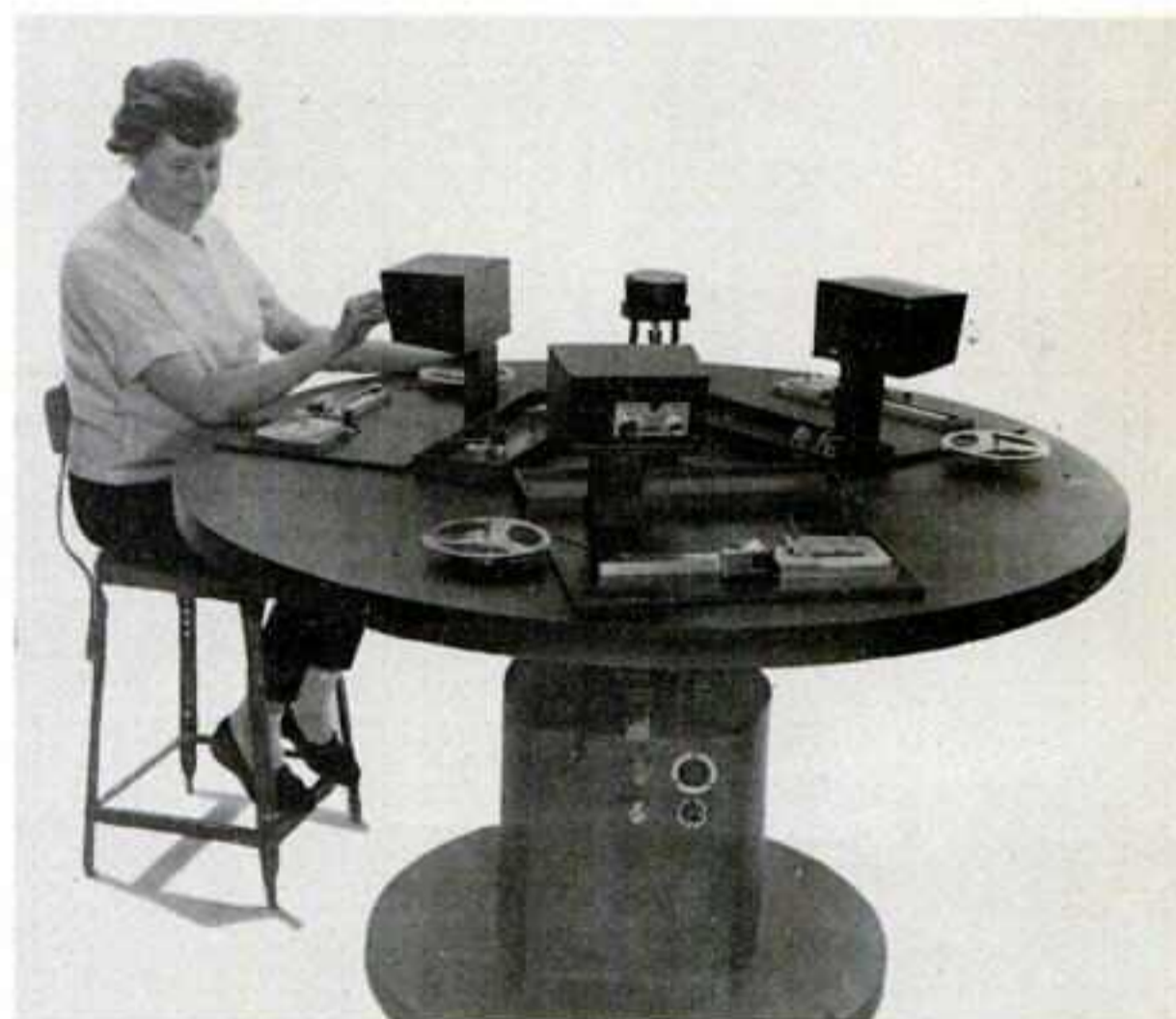
THE PACER, by Sarex Corp., loads up to 2,880 CARtridges or cassettes of 300-foot length in one shift. One operator, with no previous experience, is needed to work the rotating table, which loads at 320 i.p.s. in 10 seconds.
