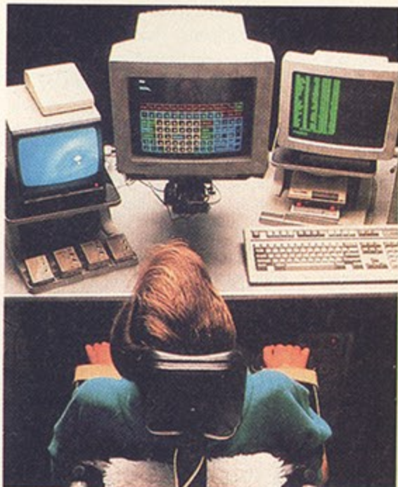
• Eventually you may only need to look at the screen to give a command. This American system tracks your eye by observing the pupil with a video camera. It is only a small step to imagine 'double-blinking' on a file to open it, or dragging a document across the screen by squinting. The system is entirely non-obtrusive.
