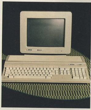
The 1224 is a medium-res colour monitor with the advantage of matching the styling of the ST.
