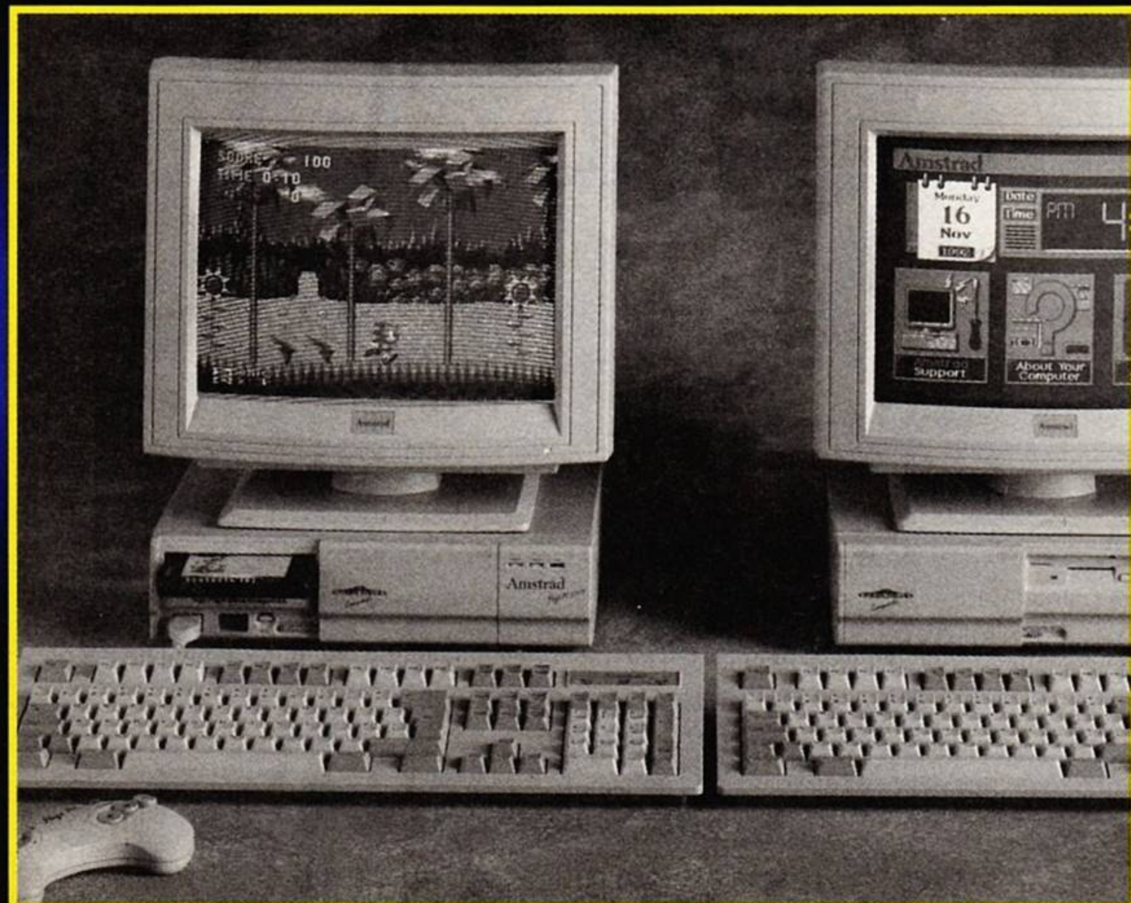
The Mega PC has a sliding panel which either uncovers the disk drive or, if you tweak it to the right, the cartridge port. Very neat design, we say.
