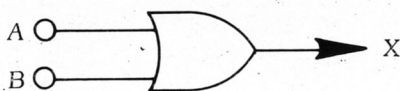
Fig. 1-5. The symbol and associated truth table for the OR gate. The function is identical to the circuit in fig. 1-4.
