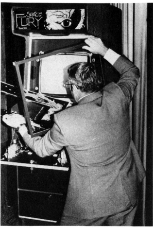
On stage, a Gremlin engineer demonstrates the conversion process. In the first photo, the screen graphics are removed and replaced. In the second photo, PC boards are interchanged. In the third photo, the control panel is exchanged. The fourth photos shows the end result—a Space Fury converted into a Battle Star. Time elapsed: 13 minutes.
