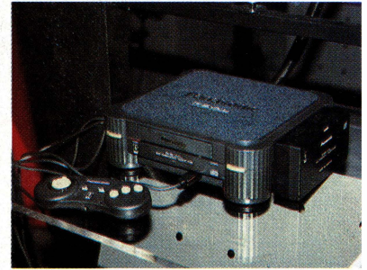
Panasonic's FZ1 digital video adaptor (above) uses the MPEG1 chipset for full-motion video
