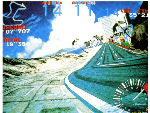
Ridge Racer's astonishing roadways are made up of texture-mapped polygons. Namco's System 22 hardware represents the state-of-the-art in 3D coin-op technology – for the present...
