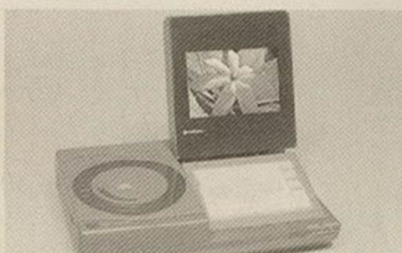
• The Hitachi CD 2 is a portable CD-ROM viewer which incorporates its own 5-inch colour TFT LCD screen.
