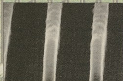
• These lines are just 0.07µm across, drawn by an electron microscope.
