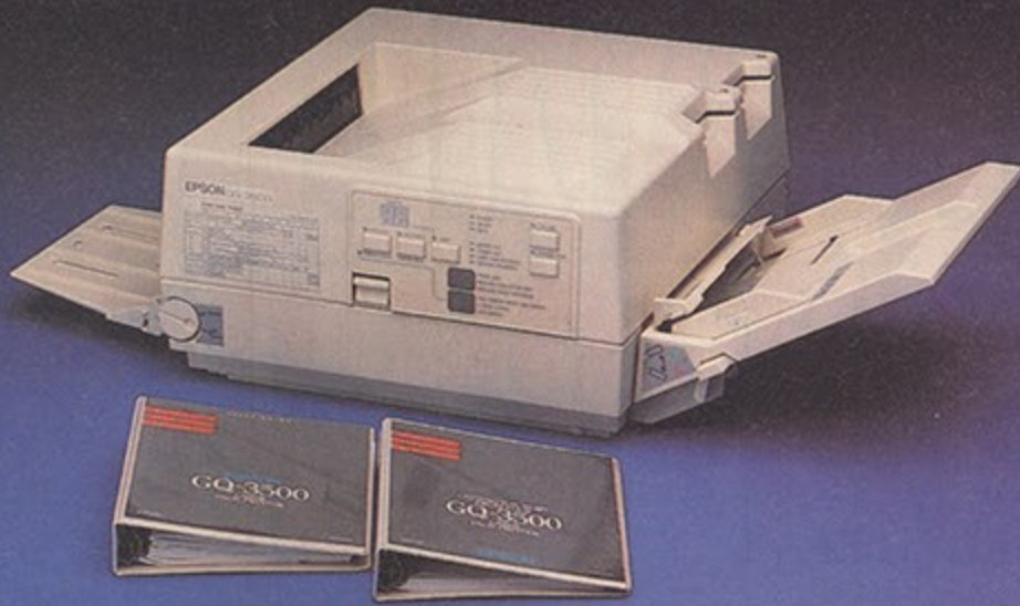
• A typical laser printer: look for Hewlett-Packard LaserJet compatibility and plenty of memory – you need at least 1.5Mb to do serious DTP work.
