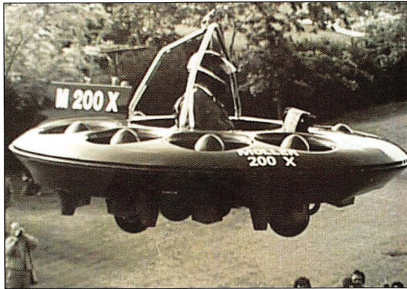
Early models (above) used go-kart engines to provide lift-off. Will the Skycar replace the Nissan Skyline GTR as the status symbol among industry players?
