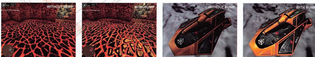
Dungeon Keeper 2 and Battlezone II are among the wealth of current games that have shipped supporting the G400's environmental bump mapping. Although it doesn't add any additional gameplay features, there's no question that it makes titles look considerably more realistic
