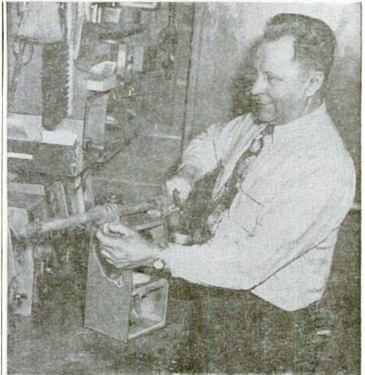
SAMP USES A MANUAL CLAMP TO CEMENT the joints on a rebuilt vending machine for his route. His immaculate machines and sparkling maintenance program are a trademark.
