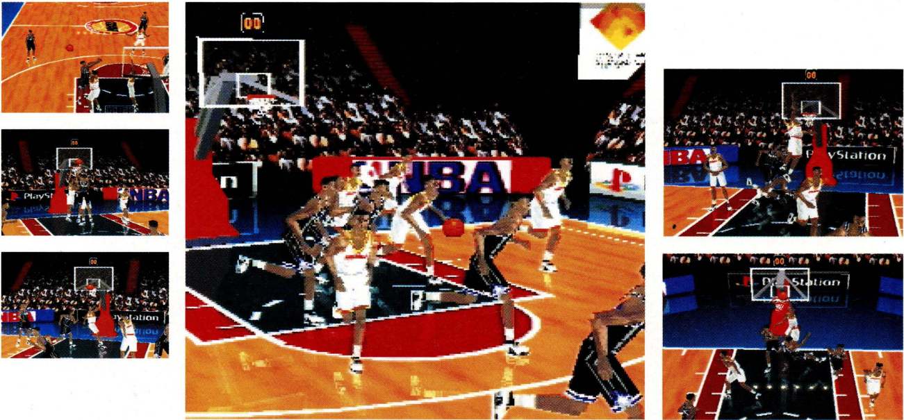
'The reflections of the static environment - features like stands, lights [bottom right], surround ad, boards, etc - are actually part of the court model. The polygons drawn are semi-transparent and, in fact, drawn on top of the floor. The reflections of the players' legs [centre] are calculated live by reversing the 3D polygons of the lower limbs of the players and drawing them on the court surface. These are real reflections' - Jules Burt, producer for SCE Europe.
