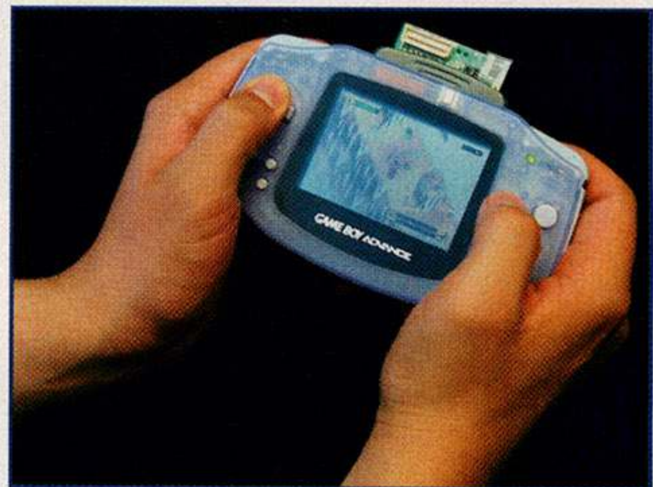
Boktai 's solar sensor sits on the upper right-hand corner of the cartridge. (The retail version will encase the sensor inside a clear cart, so it won't be exposed like this.)
