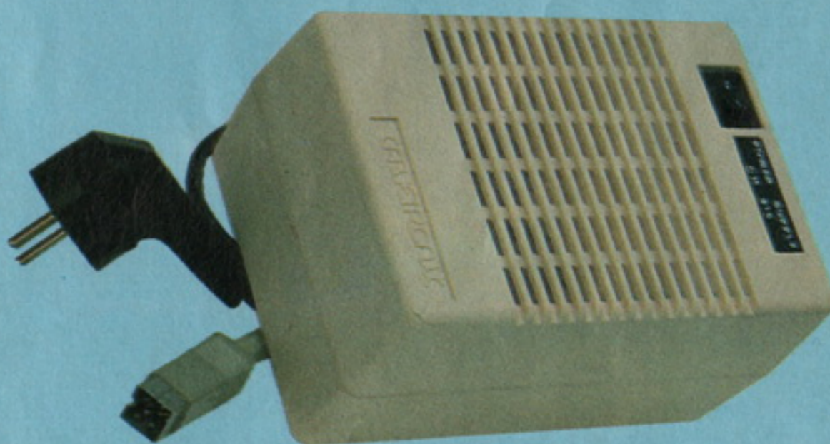
Power supply for Commodore Amiga 500. ART. CH 315. Input 220 V./50 Hz. - Output 5,1V./4A. + 12V./1,2A. - 12V./0,5A.
