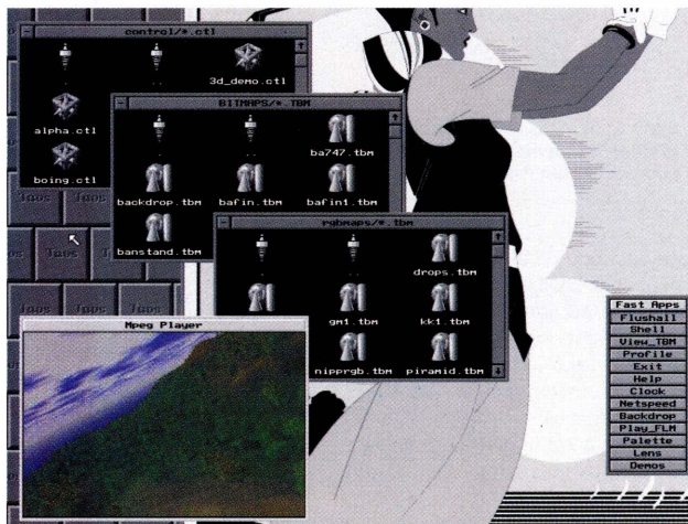
With set-top boxes in mind, Taos has support for a software MPEG player (running, bottom left) and PostScript graphics (on the right)
