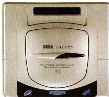
Saturn's switchgear (left to right): power on/off, CD lid release and reset button
