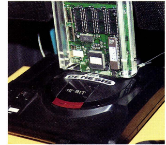
Sega's SVP chip, as used in Virtua Racing on the Mega Drive
