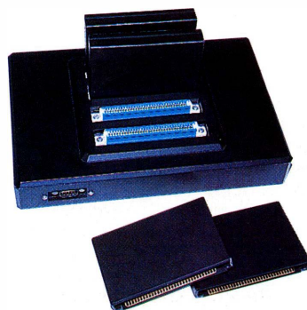
Chris built a console prototype which utilises transputer 'carts': the more you plug in the faster it runs
