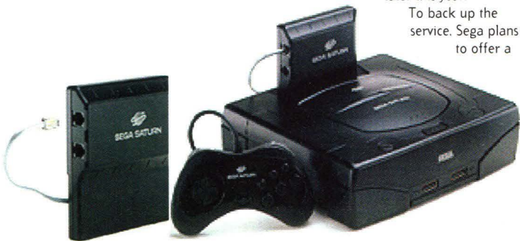
The Saturn Net Link fits into the cartridge port on the back of the console and combines a high-speed modem with a Net browser
