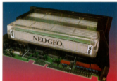
The Neo-Geo M1-FX2 is a single-slot JAMMA-standard PCB that plays Neo-Geo MVS arcade cartridges (see letter from Alan Partridge)
