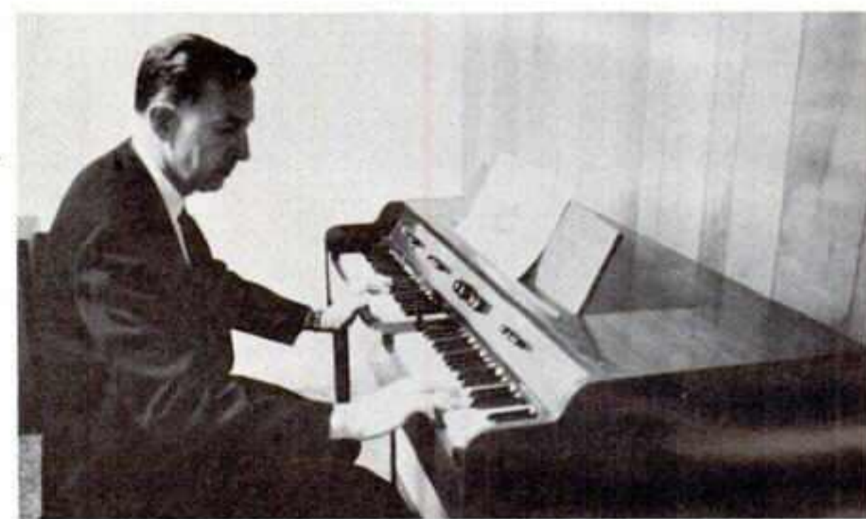
ONE-MAN BAND: Ernest Van Leeuwen, of Hollywood's Magnetic Recorders, at the keyboard of the Chamberlin Music Master. Instrument has organ-like appearance, but offers sounds of many instruments on pre-recorded tapes.
