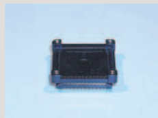
① NQPACK Connector soldered onto target system
