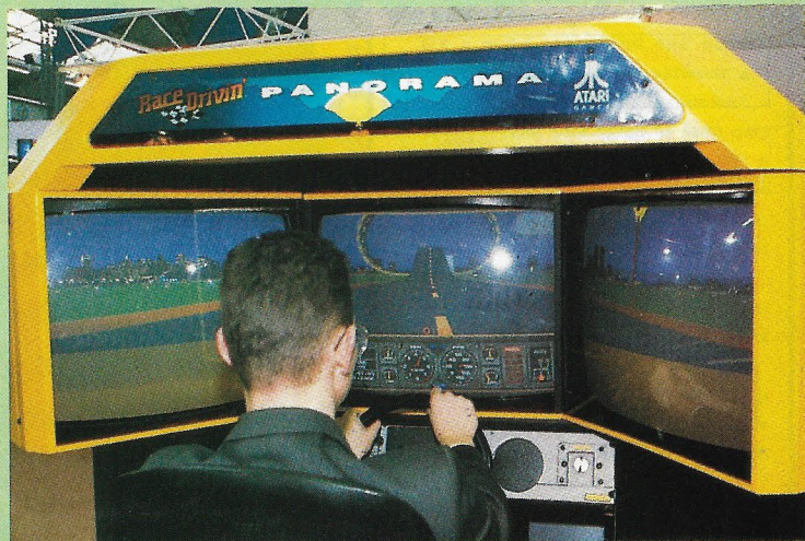
In Race Drivin' Panorama , the three monitors combine to display a 170 degree view
