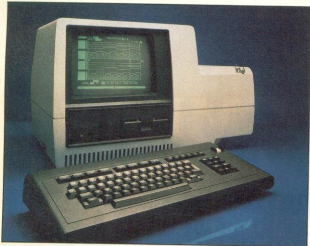
Combining hardware and software tools, the Intellec Series IV simplifies the design of products based on iAPX 86, 88, 186, 188, and 286 microprocessors.
