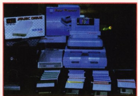
The Super Magicom transfers S-NES carts to computer disks.
