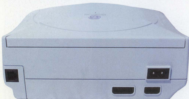
Like its Japanese counterpart, the western unit will ship with a modem, slotted into the rear-left of the console. It will be a 56K model, though
