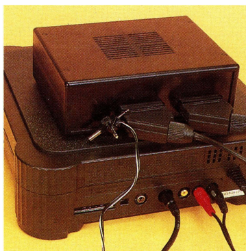
MD Consoles' S-VHS to Scart box lets you use imported 3DOs on a PAL TV
