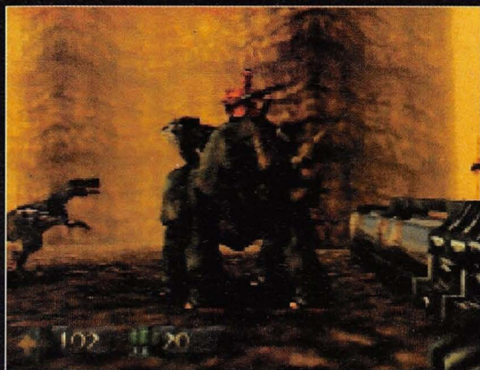
The fogging effect in Turok enables the game to reduce the poly count by ignoring objects beyond the middle distance
