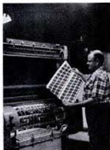
KIVAR, a special water-proof, plastic covering material, is being printed here prior to wrapping around beaverboard used in Amberg's cases.
