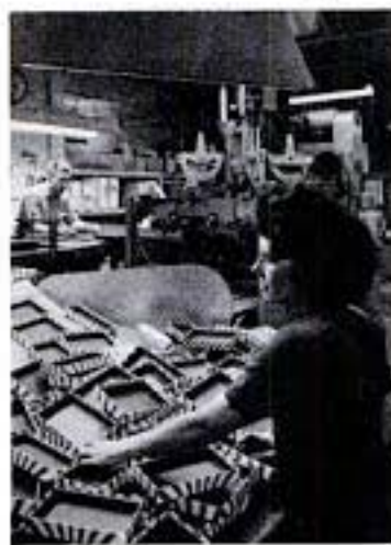
OP ART DESIGN is evident in this stage of construction at Amberg's Kankakee, Illinois plant. Here, lids of cases are being wrapped.
