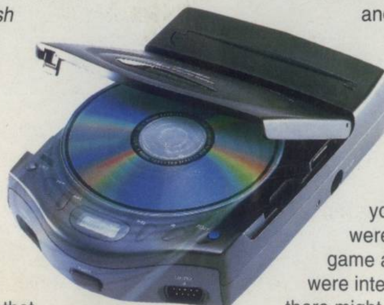
The CDX. A combined Mega Drive and Mega CD, not to be confused with the Saturn Super Console
