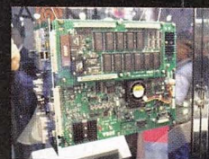
Although the board is closely related to Sega's Dreamcast, it features double the RAM (32Mb) and twice the VRAM (16Mb) of the console
