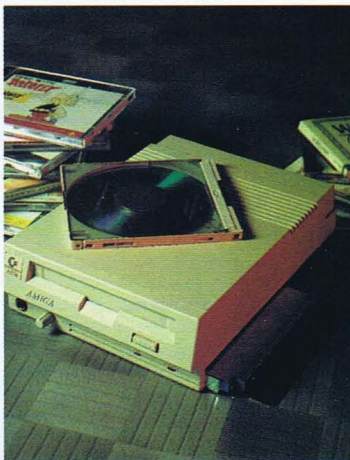
The Amiga pioneered CD as a games and multimedia format through the introduction of CDTV and devices like the A570 (above), an A500 CD add-on
