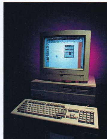
The A1500 was a SCSI-less variant of the A2000, to suit smaller pockets
