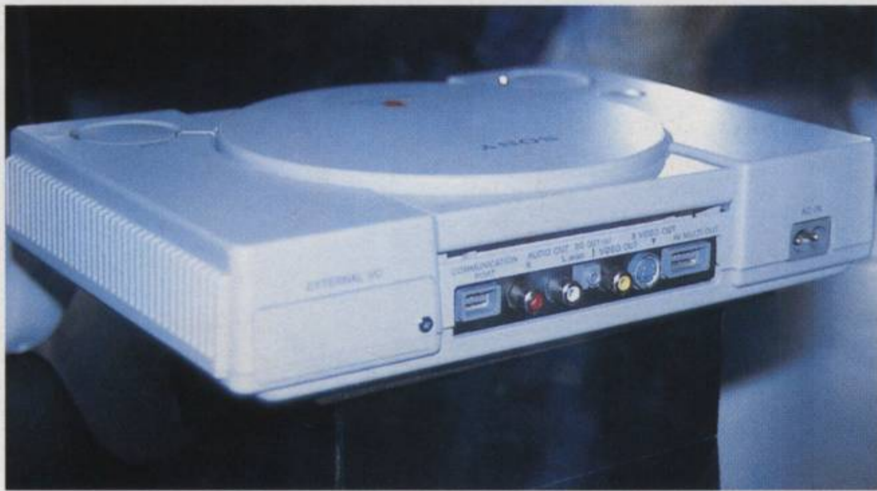
The PlayStation incorporates (from left) a comm port, stereo jacks, DC out (5V), composite video, S-Video, and an RGB AV multi-out
