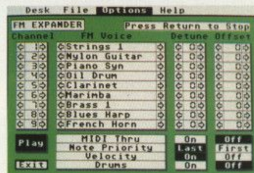
The FM Melody Maker from Hybrid Arts has plenty of options to customise the sounds. Each one can be assigned to a separate MIDI channel.
