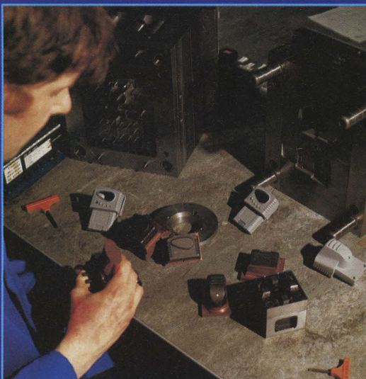
The Shockwave, like all of Datel's products, uses a plastic casing designed and moulded at its own plant
