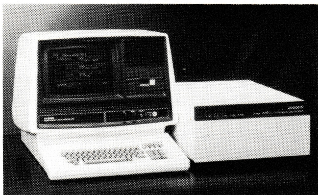
This Sord M243 Mark VI includes an optional floppy disk drive integrated into the display and the standard 8-inch Winchester disk drive, right, in a separate enclosure.
