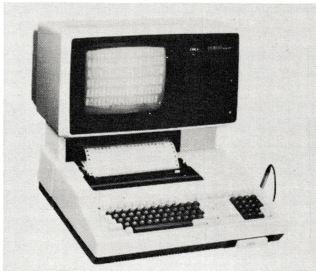
This IF800 Model 20 has a keyboard, matrix printer, 12-inch color display, two mini-floppy disk drives, and an optional light pen. Below the keyboard, at right front, there is a ROM cartridge slot.
