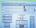
The main display for Track 24 sequencer on the Atari ST. Note the cassette recorder icons for record and playback.
