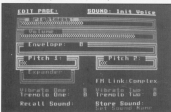
Commodore FM Sound Editor - this is the edit window, allowing you to define the characteristics of one sound - which in this package can be anything but a note.
