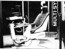
• THE KONIX HOT SEAT: A prototype of the arcade chair, driven by three electric drill motors and controlled by a joystick rather than by a Multi System game
