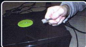
▲ Using the ethernet connection, you can daisy-chain Xboxes together for multi-player fun.
