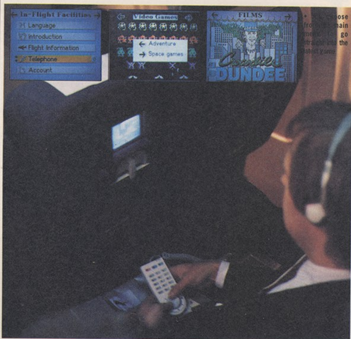
• IFESS installed - the 6.5-inch colour monitor will also come in arm and headrest formats
