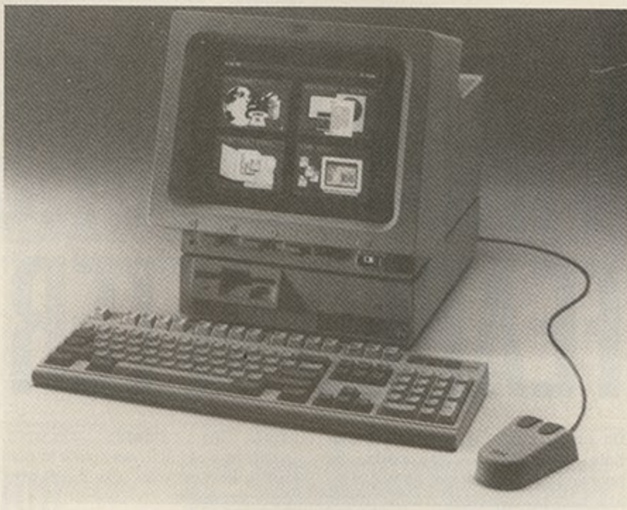
• The IBM PS/1. The co-ordinated unit takes its power from the monitor, allowing it to be controlled by a single switch. Note that there is no potential for adding a second disk drive into the main unit.
