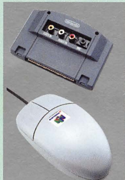
The two additional devices for use with the Mario Artist suite are the N64 mouse and the video-capture cartridge. Video-in quality is likely to be merely adequate.
