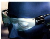
VRD uses patterns of light to create images on the eye's retina
