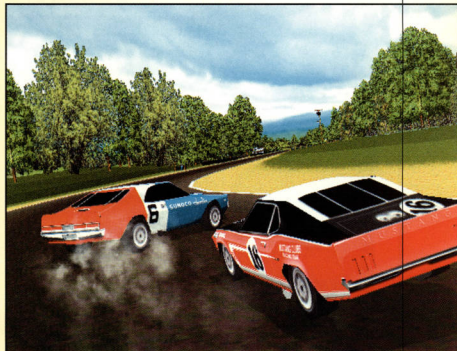
Expect the screen to refresh at a rate of 30fps. Car models average 250 polygons but can be as low as 75 and as high as 400
