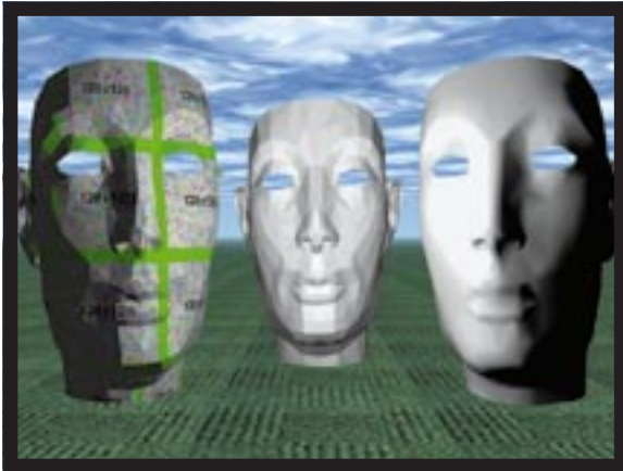
Texture mapping, lighting (point source), Gouraud shading
