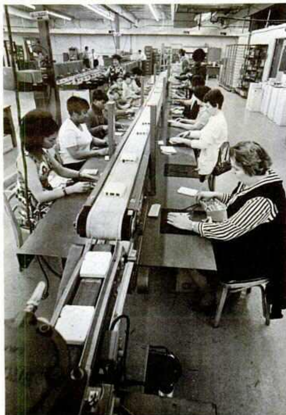
BUSY FINGERS are helped by electronically operated splicing equipment as tape CARtridges make their way along the 8-track assembly line. These units developed by Livingston Audio are available to the industry.
