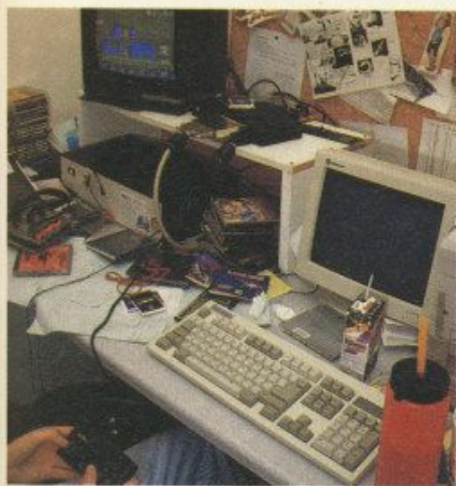
Alex's NEC development system makes developing for the machine a doddle. Well, almost. 'It's just a huge box of RAM,' he explains, 'I write the source code using a wordprocessor on a PC, compile it, and then squirt down into the box, which behaves exactly like a vast cartridge. I can then play it on the PC Engine in front of me...'
