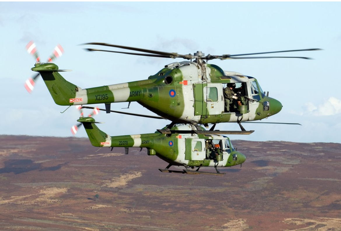
A pair of Lynx AH.Mk.7s of the AAC's 9 Regiment armed with 7.62-mm machine-guns
