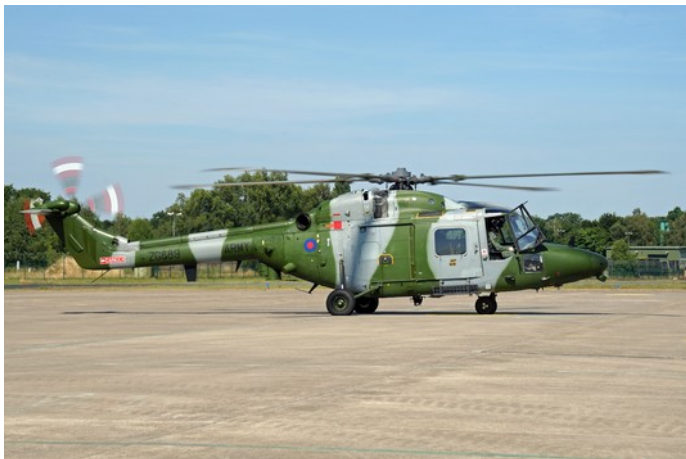
Lynx AH.Mk 9 of 1 Regt AAC with tricycle landing gear
