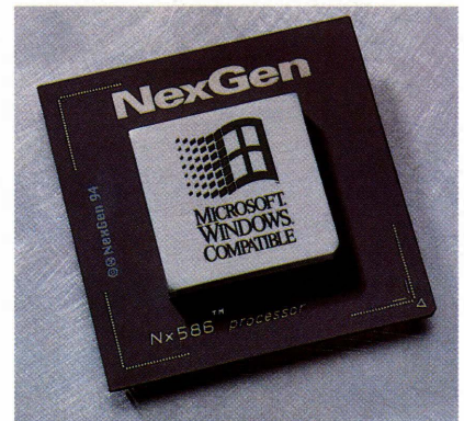
The NextGen Nx586 is one of the first of a new breed of RISC-based processors which can run Intel 80x86 code
