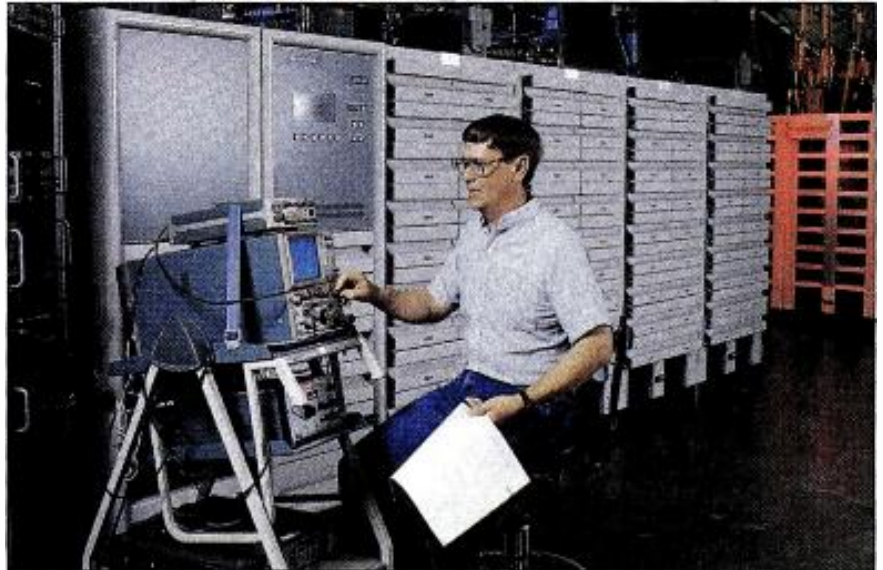
A Harris engineer tests a Platinum Series VHF solid-state transmitter.
