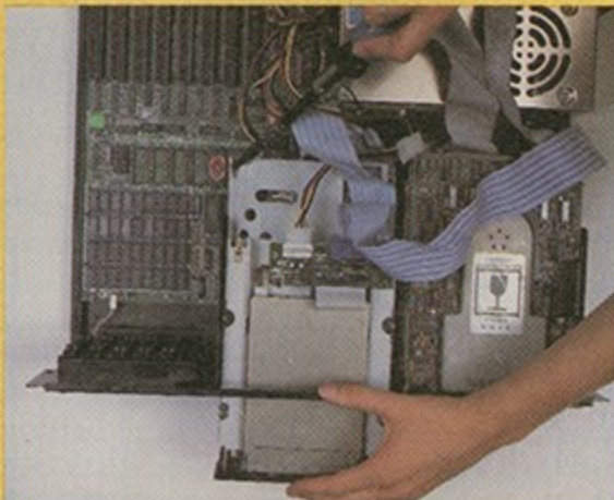
• With the expansion cards removed, the disk drives are unscrewed and slid out of the front.
